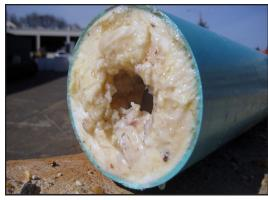
Grease coats the inside of sewer pipes when disposed of incorrectly creating sewer blockages. Often wipes are found in the grease contributing to hardening and compaction.
